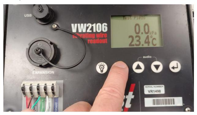
Repeat this process for each of the locations to be created in the VW2106 Readout.
