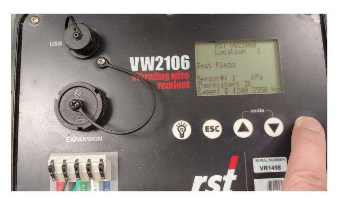
Once you have selected the location with the enter key, the 'Monitor Settings' screen will come up again. Press ESC to go back to the pressure and temperature readings.
