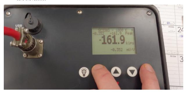
15) The load cell is now zeroed and ready for use. This can be used to reset the readout each time it is used by pressing the keys twice to toggle between offset and zero.
